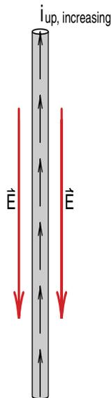
In Figure (15), we have sketched a field structure consisting of a circular magnetic field and a downward electric field that started out at the wire and is expanding radially outward at a speed  $v$  as shown. This structure has not yet expanded out to our Path (1), so that the line integral  $\oint \vec{B} \cdot d\vec{\ell}$  is still zero and Ampere's law still requires that
