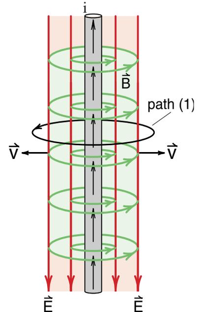
What happens when the field structure gets to and passes our path? The situation suddenly changes. Now we have a magnetic field at the path, so that  $\oint \vec{B} \cdot d\vec{\ell}$  is no longer zero. And now the expanding front is outside our path so that the expansion no longer contributes to  $-d\Phi_E/dt$ . The sudden appearance of  $\oint \vec{B} \cdot d\vec{\ell}$  is precisely compensated by the sudden loss of the  $d\Phi_E/dt$  due to expansion of the field structure.
